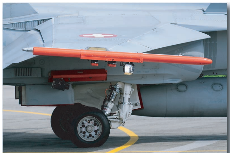
Camera racks attached to the weapons hard points. In this instance to record modifications to the landing gear. Various camera outfits could be carried. Check www.mc-one.ch for more information.
